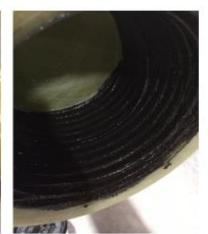
Start the engagement of threads and tighten by hand until snug; pipe should turn freely with minimal friction, if properly aligned. Then use the backup Wrench on the Female side. Set the torque Wrench to 600 Ft/lbs and complete the makeup. Note: No threads exposed.
